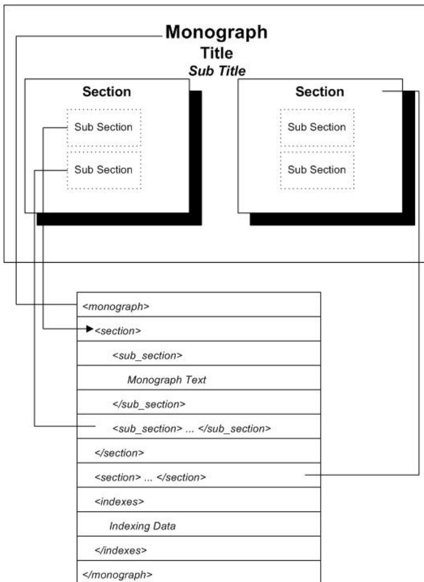
**Figure 5. Common Object XML Mapping**
